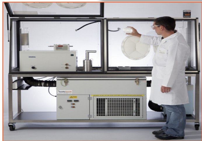
The hand built air treatment unit sits at the core of the ClimateZone operation, regulating both temperature & humidity.
